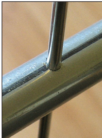
Figure 8 — Close-up of boom dimpling.
