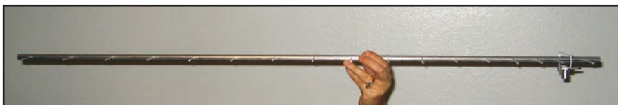
Figure 16 — Side view of the finished Yagi. Note the element alignment
