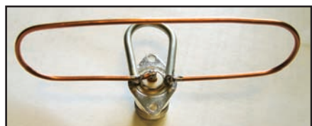
Figure 12 — Another view of the completed driven element.
